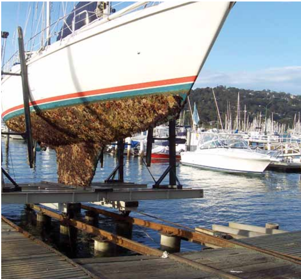
A heavily biofouled yacht being slipped for a clean and antifouling paint renewal.
