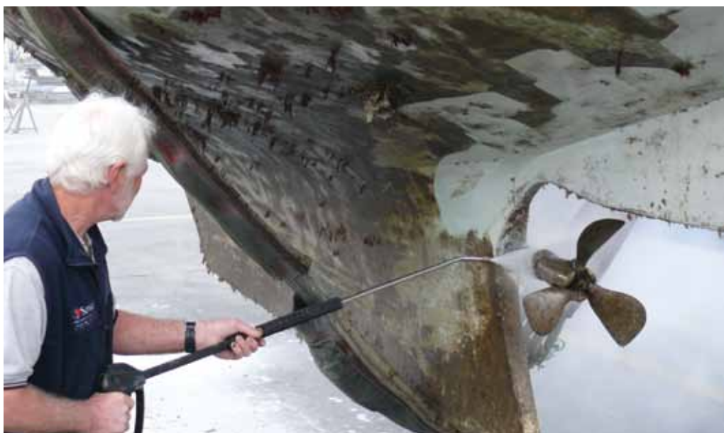
Biofouling on a recreational vessel being removed by hydroblasting.
