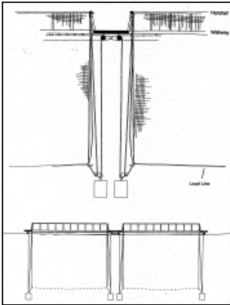
**Figure 7 Example of net tensioning using individual pulley weights (from Arnold 1992)**
